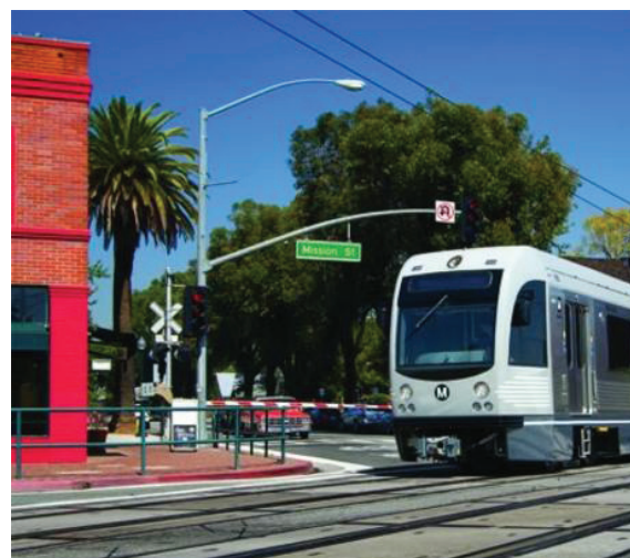
Gates and pedestrian arms are common types of safety elements for pedestrians at rail crossings.
