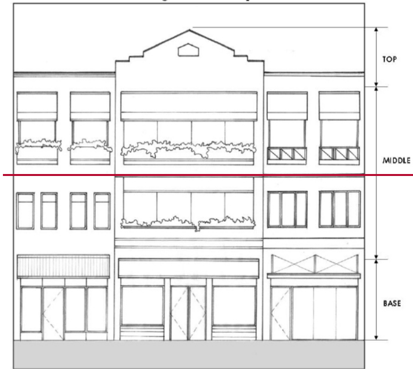
Figure 4-6 Building Elevation Composition
