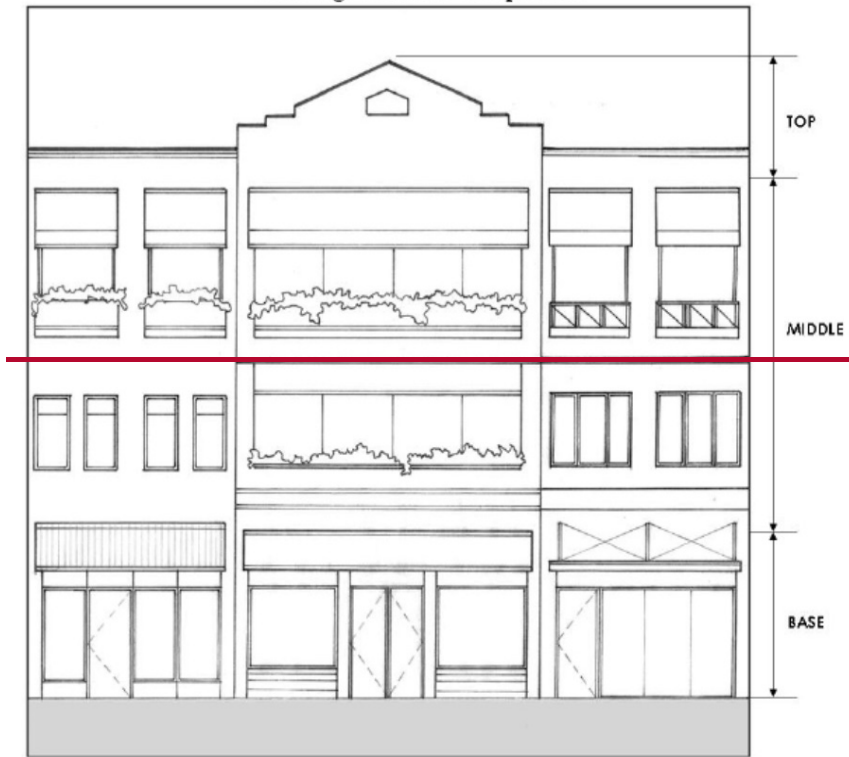
Figure 4-6 Building Elevation Composition
