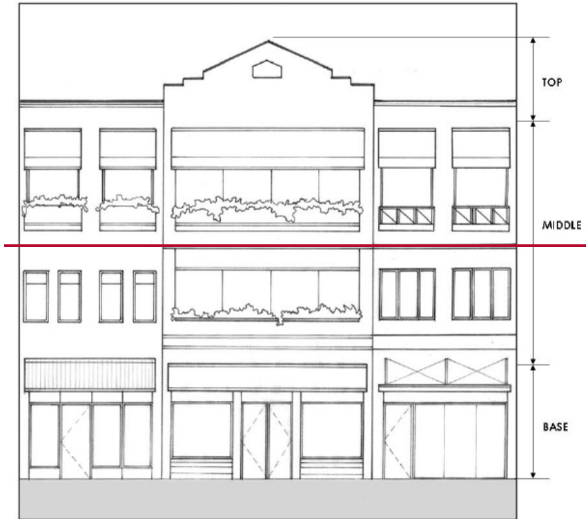
Figure 4-6 Building Elevation Composition
